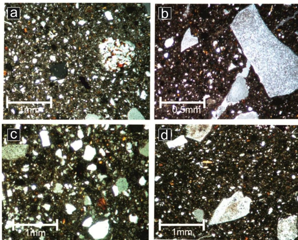
Figure 4. Crossed-nicols microphotographs of laboratory tests fired at 900°C: (a) CORFU1-10S; (b) CORFU2-10S; (c) CORFU3-10S; (d) CORFU4-10S.
