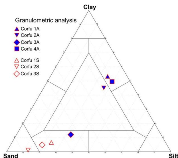
Figure 3. Grain-size classification according to Sheppard's diagram for the sediment sampled in Corfu (CORFU1A-4A and CORFU1S-3S).
