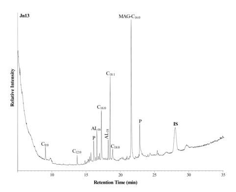
Figure 2. Partial (0-35 min) total-ion-chromatogram (TIC) of the trimethylsilylated total lipid extract of the organic residue obtained via conventional solvent extraction from the interior of sherd Jn13. ( $C_{x:y}$ ): monocarboxylic fatty acid of carbon chain length x and degree of unsaturation y, (MAG- $C_{x:y}$ ): monoacylglycerol with  $C_{x:y}$  fatty acid moiety, (P): plasticizer, and (IS): the internal standard (n-tetratriacontane;  $C_{34}$ ).
