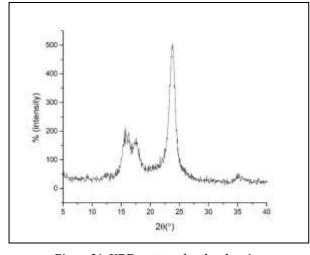
Figure 21. XRD pattern for the cleaning method with Wolbers solvent acetone gel crystallinity index=61.4 showing a slight increase in the crystallinity index in the cellulose crystallinity compared to the control sample which means that a moderate change has occurred in the chemical and mechanical properties of cellulose molecule
