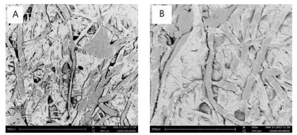
Figure 4. SEM micrographs of paper sample; Photo A shows the paper support after cleaning with hydro gellan gel prepared in the lab. B shows the paper support after aging.
