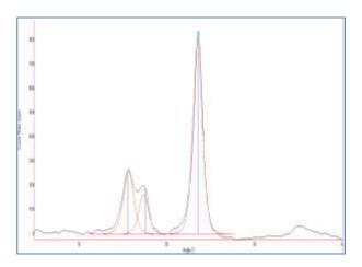
Figure 16. X-ray diffraction pattern of historical paper sample explaining how the crystallinity peaks of cellulose are measured
