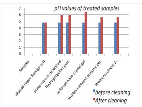
Figure 14. pH values of untreated & treated paper samples.
