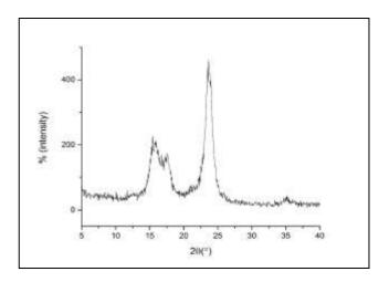
Figure 18. XRD pattern for the cleaning method with akapad paper sponge Crystallinity index=11.16 showing a large decrease in the crystallinity index of cellulose, indicating that a significant change has occurred in the chemical and mechanical Properties of cellulose molecule.
