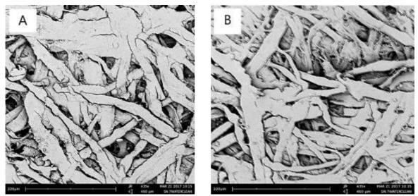
Figure 2. SEM micrographs of paper sample after cleaning with deionized water; photo A show the paper surface after cleaning treatment while B show the paper Surface after aging. (wet cleaning)
