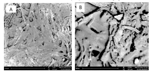
Figure 7. SEM micrographs of paper sample Photo A shows the paper support after cleaning with Wolbers Solvent gel isopropanol while B shows the surface after accelerated thermal ageing.
