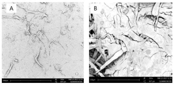
Figure 5. SEM micrographs of paper sample; Photo A shows the paper support after cleaning with Cellulose Nano Crystal gel prepared in the lab, this method was performed in order to clean and consolidate paper while B shows the surface after accelerated thermal ageing.
