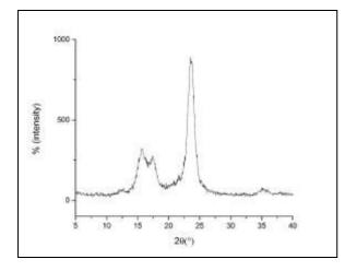
Figure 17. XRD pattern for the cleaning method with deionized water crystallinity index=11 showing a large decrease in the crystallinity index of cellulose indicating that a significant change has occurred in the chemical and mechanical properties of cellulose molecule.
