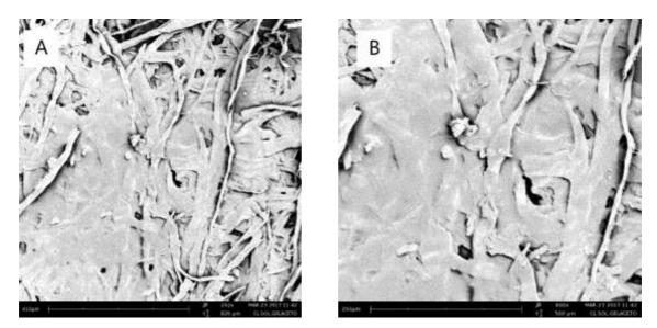
Figure 6. SEM micrographs of paper sample; Photo A shows the paper support after cleaning with Wolbers solvent gel acetone while B shows the surface after accelerated thermal ageing.
