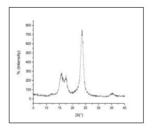
Figure 19. XRD pattern for the cleaning method with hydro Gellan gum crystallinity index=58.3 showing a slight decrease in the crystallinity index of cellulose indicating that only a less change has occur the chemical and mechanical properties of cellulose molecule.
