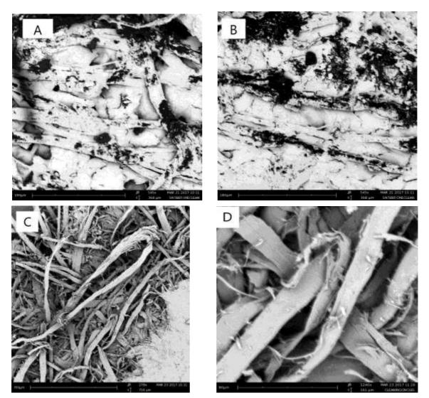
Figure 1. SEM micrographs of historical sample before and after cleaning methods.; Photo A and B show critical damage of paper support while C,D show SEM image of cotton fibres used to make the paper support.
