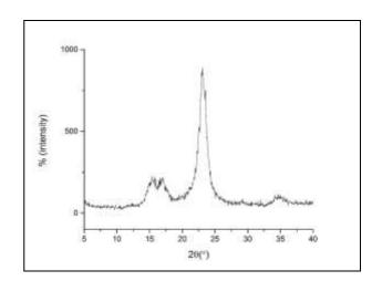
Figure 20. XRD pattern for the cleaning method with Cellulose Nano Crystal gel crystallinity index=17.00 showing a large decrease in the crystallinity index of cellulose, indicating that a significant change has occurred in the chemical and mechanical properties of cellulose molecule at the crystalline regions.
