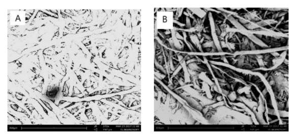
Figure 3. SEM micrographs of paper sample ;Photo A shows the paper surface after cleaning with akapad soft sponge the sponge works by absorbing dirt particles, then crumbling of to avoid polishing the treated surface while B shows the cellulose fibre after ageing . (Mechanical cleaning)
