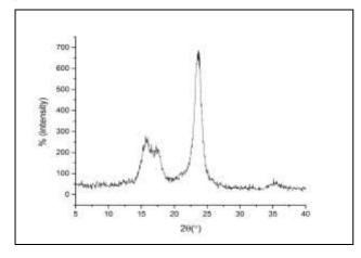
Figure 15. XRD pattern for the control sample before cleaning Crystallinity index=61
