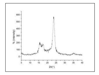
Figure 22. XRD pattern for the cleaning method with Wolbers solvent 2-propanol gel crystallinity index=18.5 showing a large decrease in the crystallinity index of cellulose, indicating that a significant change has occurred in the chemical and mechanical properties of cellulose molecule at the crystalline regions
