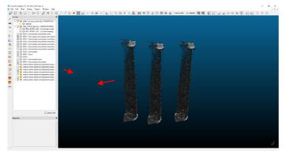
Figure 26. Abstracted columns to be aligned
