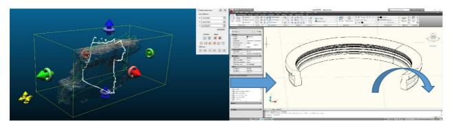
Figure 29. Export cross-section to CAD(eg DXF). Identify Radius and Arc. Revolve Cross Section (Autodesk - AutoCAD 2015)
