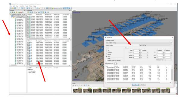
Figure 16. Loading Images, GCP's and image position/orientation to photogrammetry software. Note the difference of reference system between GCP and Images
