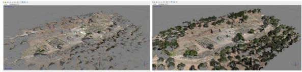
Figure 18. Sparse Point cloud generation and GCP'S (303.436 Points).
