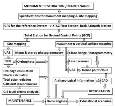
Figure 1. Diagram for restoration and maintenance.
