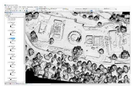
Figure 34. Hill shade relief with shadows visible form the beginning (light grey) to end (dark grey) of Sites working hour.
