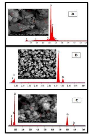
Fig. 3 SEM micrographs and EDX analysis of nano-materials A) Ag, B)TiO<sub>2</sub>, C) CuO
