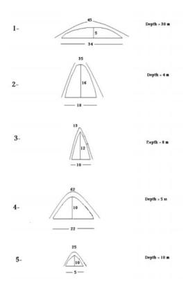
Figure 8. The dimensions of some of the quarries
